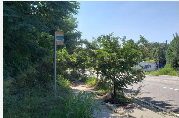
Figure 12 | Example of a bus stop hidden by excessive foliage, and where riders would need to lean into the roadway to flag the bus down.
